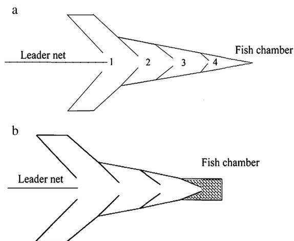
Figure 1. Basic design for set traps for salmonids; (a) salmon trap, (b) combi trap, and combiD trap.
