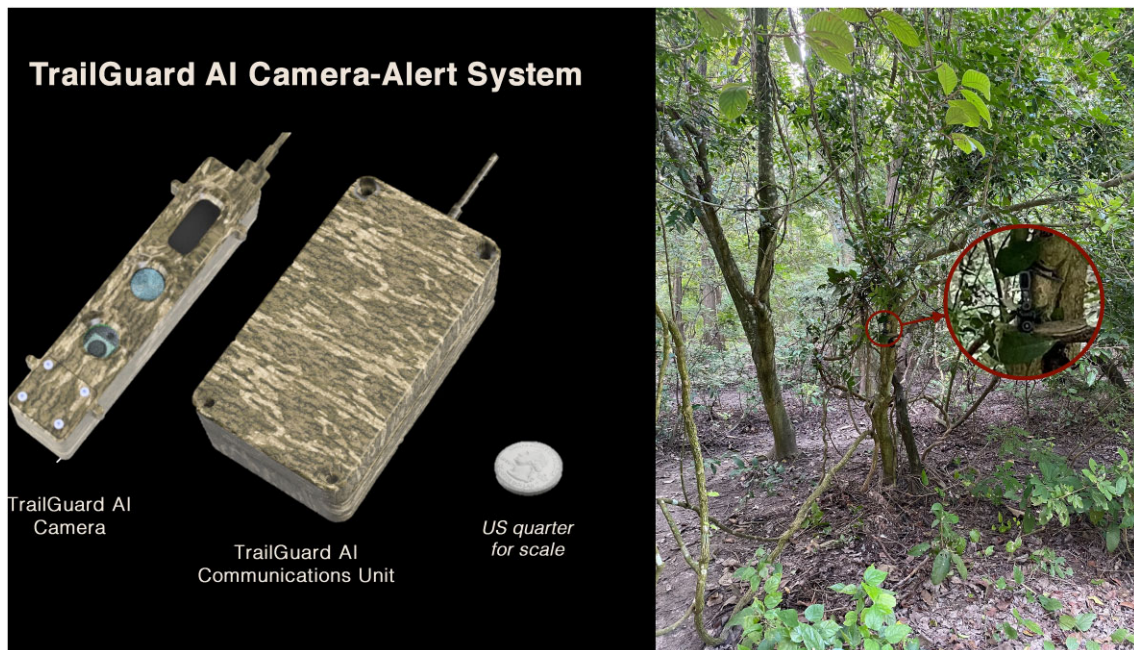
Figure 2. The TrailGuard AI camera system (left, US quarter for scale) can be well camouflaged near a trail such as this one in Dudhwa Tiger Reserve, as seen from the trail, that sent multiple real-time notifications of poachers without being detected (right).
