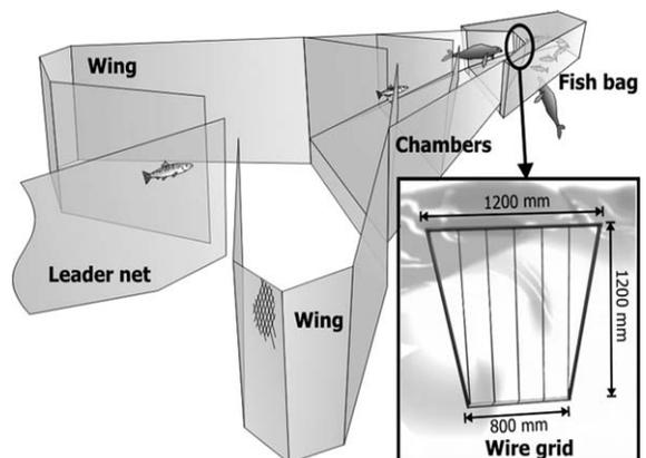
Figure 1. A salmon and whitefish trapnet equipped with a wire grid in the funnel of the fish bag. The grid is made of vertical 2-mm steel wires and its buoyant frame is constructed of stainless steel.
